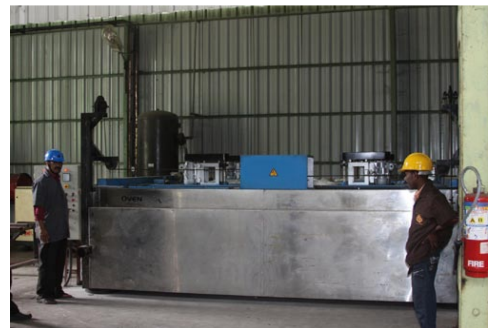
With over 500 cubic feet of working volume, it is no problem for ultra-large parts to fit into our post-curing oven that will reach temperatures up to 300° Celsius.
