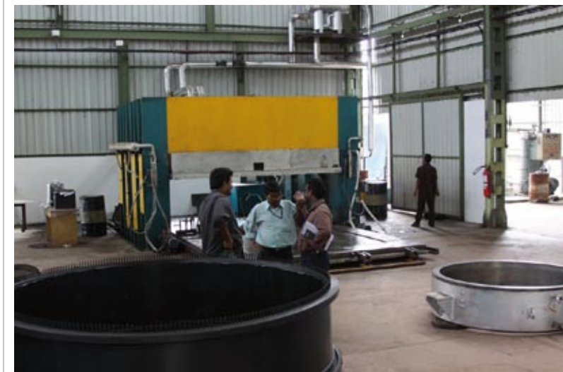
Our Indian Engineering team discusses the next steps for post-curing and inspection of the large valve seat recently molded.
